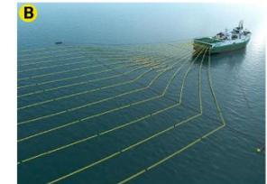
Offshore seismic survey
