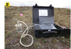
Soil gas CO<sub>2</sub> concentrations measurements
