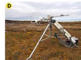
Eddy covariance towers to measure atmospheric CO<sub>2</sub> concentrations downwind of a leak
